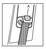
To move it down, press the release button (A) and move the height adjuster to the desired position. You can move the height adjuster up just by pushing up on the shoulder belt quide.
